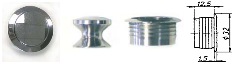
Drill hole 26 mm diameter for ring #24.552 button and #24.553 ring
