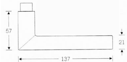
Glass door latch #82.511 with lever #11.1341; 125 mm overall; extend 25 mm or 1 inch from surface
